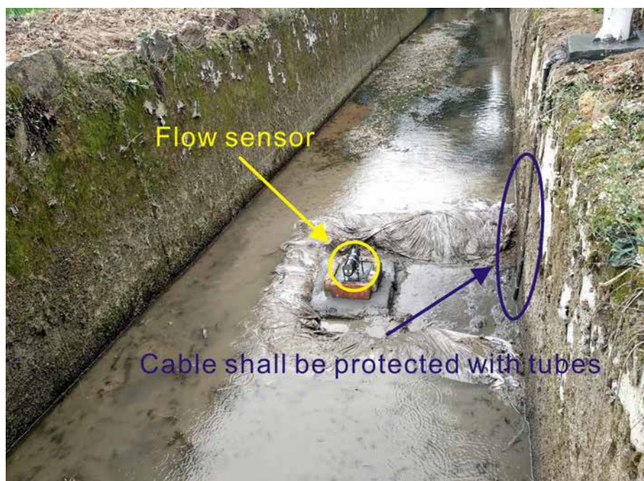
Fig. 27 Installation Mode for Channels with Silt Deposit
