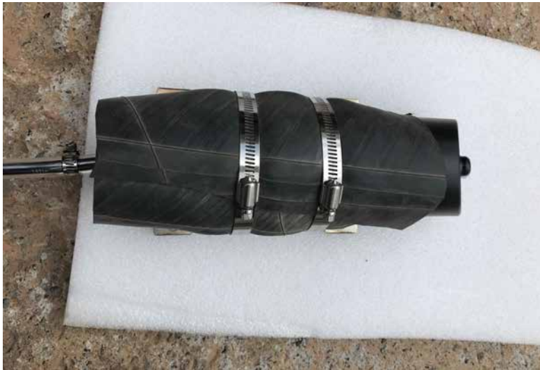
Fig. 32 Wrapping up Sensor with over 2 mm-thick Rubber Cover
