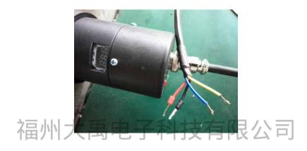
The power cord: 24 v + red line; GND by black line Current: the current + take the blue line; Current - pick up the yellow line 485 Communication output::A, pick up the yellow line. B take the blue line
