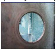
2)put A sheet of same inner diameter of gasket on the flange
